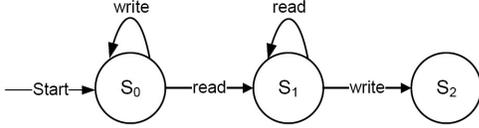
**Figure 2.** State machine tracking an observed field’s stationarity. If the final state is  $S_0$  or  $S_1$ , the field is considered stationary. Once the state becomes  $S_2$ , the field is determined non-stationary and the instrumentation tracking its status can be removed.
