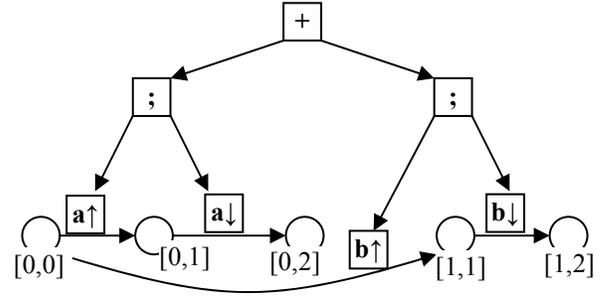
Fig. 3. Generating states and transitions of PTA. Circles represent states. Squares represent nodes of PT.
